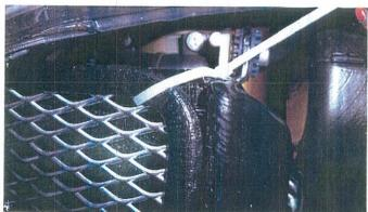
2. Place the Guard in front of the oil cooler and then feed the cable ties through the guard and the radiator core to attach. Do this in each corner.
