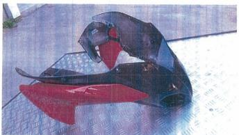
1. Remove the nose cone from the bike. This comes off nice and easily in one piece once.
