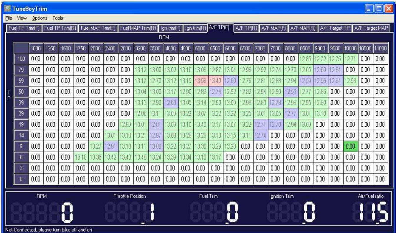
In the image above you can see that most points in the map are green. The text colour is grey to indicate that changes have been made, based on these readings. The few points that still show red and blue have had a correction made based on these values. If the bike was run through these points again the values should be on target. In effect this screen shot shows the second to last state of tune. It is not necessary to run through again as we can see the A/F values are very good.
