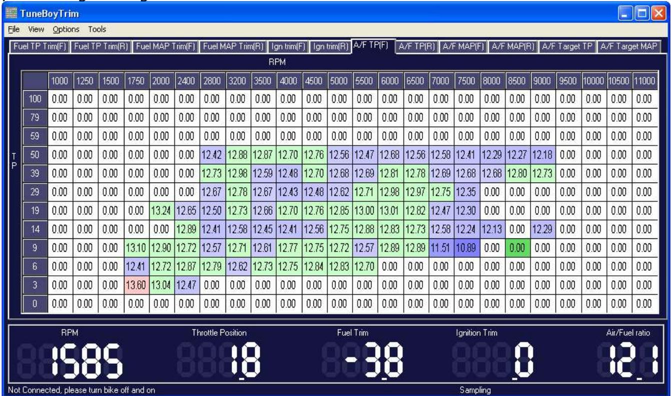
5. Now with the A/F tables filled in you can select the areas that need correcting and hit the **C** key on the keyboard to correct the fuel trim table.
